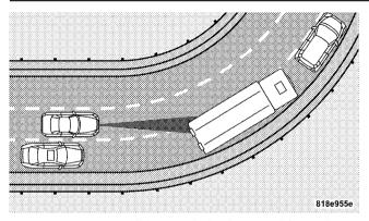
ACC may occasionally provide braking and/or a driver alert that you consider unnecessary. This may be the system's response to signs, guardrails, and other stationary objects in a curve. This may also occur at the base of steep hills. This is normal operation and your vehicle does not require service.
